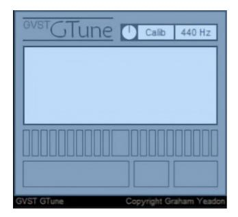
GTune guitar tuner can be used for guitar and bass tuning or for tuning other monophonic instruments such as flutes, violins, and synthesizers. This effect does not alter audio in any way.
