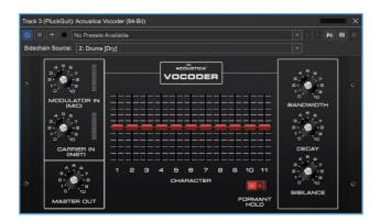
A vocoder is a specialized type of multi-filter bank that imparts the tonal characteristics of one sound upon another. Vocoders are commonly used to create robot voice or choir effects by imparting the spectral character of a spoken or sung source (aka, the "modulator") to a full-spectrum constant tone (aka, the "carrier").
