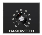
Sets the width or "Q" of all bandpass filters. Narrow bandwidths let less audio through, whereas wider bandwidths let more audio through for a denser sound. A good analogy would be to imagine water running through a comb with wide or narrow teeth.
