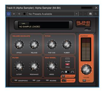
Alpha Sampler is an easy-to-use basic sampler that's fast and fun. It's so easy, it almost doesn't need any instructions; just drag an audio clip into the sample display window and play! Alpha Sampler lets you load one sound that can be played up and down the keyboard, but it's polyphonic, so you can play as many notes as you like. Alpha Sampler is included with all versions of Mixcraft.
