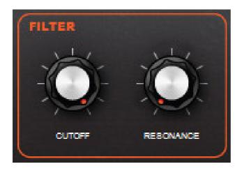
If you've ever played with filter controls on an analog synthesizer, this should be familiar; Alpha Sampler's filter is a modeled classic lowpass filter.
