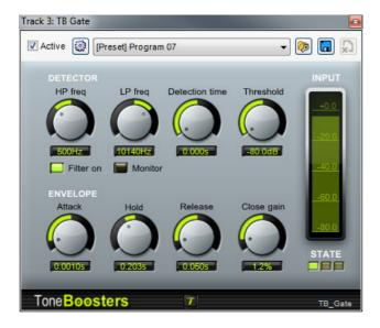
TB Gate is a very functional and simple to use gate. With its attack, hold and release parameters it can accommodate almost any gating requirements.
