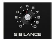
This adds high-passed white noise into the final signal when S sounds are detected. This helps speech intelligibility, because vocoders aren't inherently good at detecting S sounds, and many carrier sources don't have much energy in the S sound spectrum.
