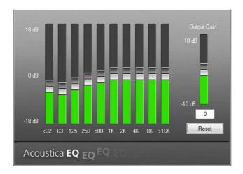
Acoustica EQ is a ten-band graphic equalizer that allows boosting or cutting of audio frequency regions. If a recording sounds thin, bass frequencies may be boosted. If a recording sounds too bright, high frequencies can be reduced. The Output Gain control is used to raise or lower overall volume after EQ processing.
