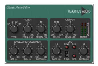
Produces filtering effects that change over time, most commonly used for automated "wah-wah" effects. However, Auto-Filter's extensive parameters allow many more musical variations including triggered effects (where the filter follows the dynamics of a sound) or synced LFO effects (where the filter opens and closes at note values locked to the project tempo).
