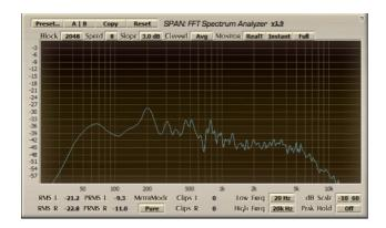
Voxengo Spectrum Analyzer is a supremely powerful tool for viewing the frequency spectrum of audio content. This is great for learning about audio frequencies and refining mixes. (Voxengo Spectrum Analyzer needs to be currently viewed to use it, so remember to click the Edit button in the Effects List or double-click the channel's FX button.)
