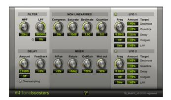
The TB MultiFX plug-in is a seriously capable effects processor! In addition to flanging, chorus, phasing and other types of mod effects, it can also do tons of delay, filter, decimation, and bit reduction effects, in all manner of combinations.
