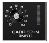
Use this to set the input level of the carrier input signal so it nominally sits in the full green/occasionally yellow region. This one **will** distort if the input is too hot, and probably not in a desirable way.
