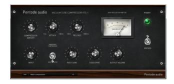
Pentode Audio VTC-1 Vacuum Tube Compressor is an analog-modeled virtual VST compressor with a warm analog and transparent sound. Compared to modern compressors, Pentode Audio VTC-1 operates differently: VTC-1 doesn't have a threshold knob; the amount of compression is set by increasing or decreasing input level as with old analog tube compressors. The Compression amount knob is similar to the ratio knob on modern compressors.
