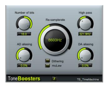
Recreate the sound of 8-bit video games, 12-bit samplers, or trash audio by transforming it into 2-bit noise! TimeMachine simulates the effect of A/D and D/A aliasing, re-sampling, and bit reduction (both linear and mu-Law quantization).
