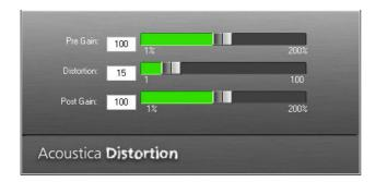
Acoustica Distortion adds audio distortion similar to that used on electric guitars. This effect can range from subtle grit to extreme destruction of the original audio. Note that adding distortion can severely affect the volume of the recording. A little distortion goes a long way, so experiment with very low settings to see how the audio is affected and increase the amount gradually.
