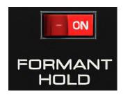
When the Formant Hold switch is on, MIDI sustain pedal messages will "freeze" the current positions of the carrier bandpass filters. This is useful if you're speaking/singing into it, and you'd like a chord to sustain its current tonality curve for long durations (as opposed to speaking/singing until hyperventilation occurs.
