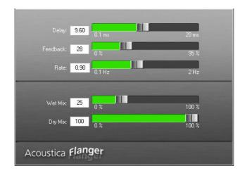
Flangers delay the signal by a small amount while slowly varying the delay time, producing a swept comb-filter effect, commonly referred to as a "jet swooshing" sound (because of its similarity to the sound of a jet plane flyby).
