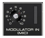
Use this knob to set the input level of the modulator signal. The bar meter should be set as with any other input level VU meter - keep it in the green
