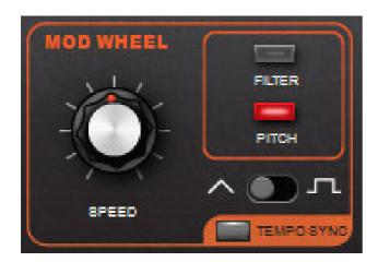
Consists of a low-frequency oscillator (LFO) capable of controlling Alpha Sampler's pitch or filter cutoff frequency, resulting in vibrato, wah wah effects, and more. One good way to think of a modulation LFO is a "third hand" to automatically turn controls up and down.
