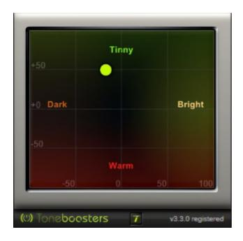
There's no easier way to EQ tracks! Instead of adjusting numeric parameters or spinning virtual knobs, EZQ lets you move a dot within a 2D plane to quickly impart brighter, darker, warmer, or tinnier sound characteristics.
