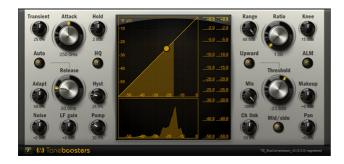
TB Bus Compressor is a full-featured stereo bus comp that can be used for glueing together completed mixes, subtly (or not subtly) crushing drum busses and more. Its extensive graphical displays offer plenty of visual feedback.
